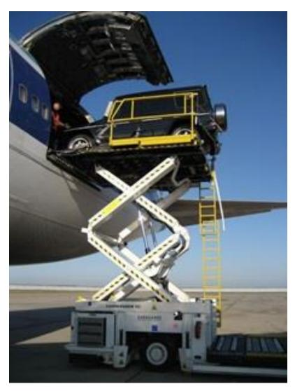
Converting your lower-deck Commander® loader to main deck height allows service of a wider range of aircraft, adding flexibility to your operation without the cost of new equipment. Upgrade features:
