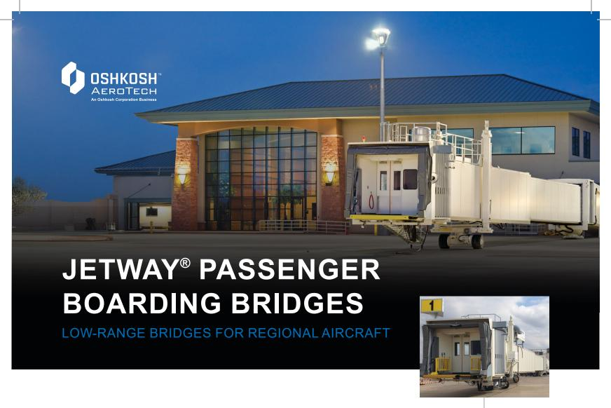
Passengers deserve the same premium large jet experience, even when traveling on smaller regional aircraft. Our low-range of passenger boarding bridges serve regional airports with standard or lower terminal floor heights. The bridge cab design is capable of negotiating doors, steps and handrails of many regional aircraft.
