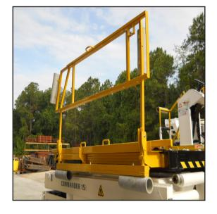
problem. By redesigning the handrail pivot point and adding a counterweight, lifting and lowering the forward bridge folding handrail becomes simple. The heavy-duty design weight of the handrail is offset by the counterweight, resulting in almost effortless lifting. When lifting from the folded-down position, only about 5lbs (22N) of lifting force is required to raise it. Specially designed, heavy-duty, tension clamps secure the handrail in
