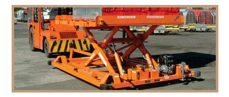
The towed Trojan Tactical Loader is designed to interface with pallet dollies, K-Loaders, C-130, C-235, C-295, C-27, Mil-8 and other aircraft. With a maximum payload of 10000 lbs (4545 kg), a tow speed of 12 mph (20 kph), and a fully powered load platform, the Trojan loader is an ideal, cost-effective cargo transfer option.
