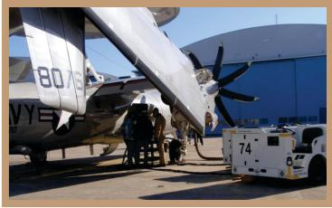
The driveable unit, with a 13 foot (4m) turn radius is ideal for operation in tight spaces and with electric drive is suitable for hangar applications. It comes with integral cable storage areas and semisolid tires and is rated for land and shipboard use. SMEPP is air-transportable on C-130, C-17, C-5, and CH-53 aircraft.
