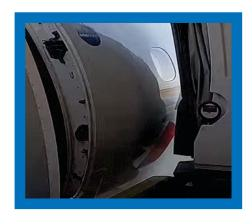
This is a \$100k to \$500k expense waiting to happen. A boarding bridge docked without the auto-level wheel deployed. iOPS from JBT can detect and notify you of these types of errors – before they become expensive problems.
