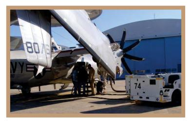
This driveable unit, with a 13 foot (4m) turn radius is ideal for operation in tight spaces and with electric drive is suitable for hangar applications. It comes with integral cable storage areas and semi-solid tires and is rated for land and shipboard use. SMEPP is air-transportable on C-130, C-17, C-5, and CH-53 aircraft.
